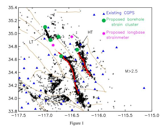
transients related to slip at these points. With installations of three instruments each at the north end of the Landers rupture, both ends of the Barstow zone, and one end of the Hector zone, we would have a monitoring capability to test for the long-term slip on these seismically active segments.
