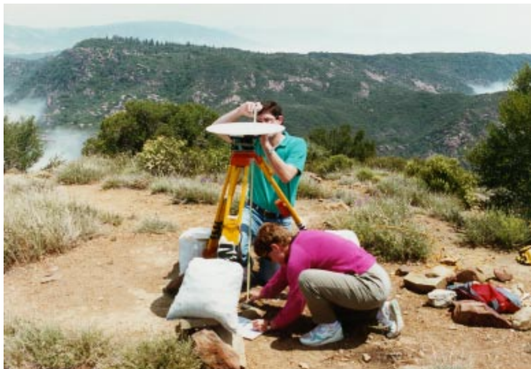
Setting up a GPS station, and measuring antenna height and reference to the monument. (Hager, left; Donnellan, right.)
