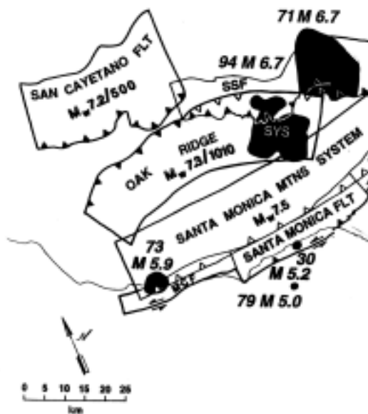
Above: Map showing the location of the San Cayetano fault, with relation to the Santa Susana (SSF), Oak Ridge, Santa Monica Mountains and Santa Monica faults. The barbs point down dip on the faults. Dark spots indicate the geometry of recent ruptures. The likely maximum magnitude event and its recurrence interval is indicated for each fault. (Figure modified from Dolan et. al, Science, 267, 199-205, 1995)
