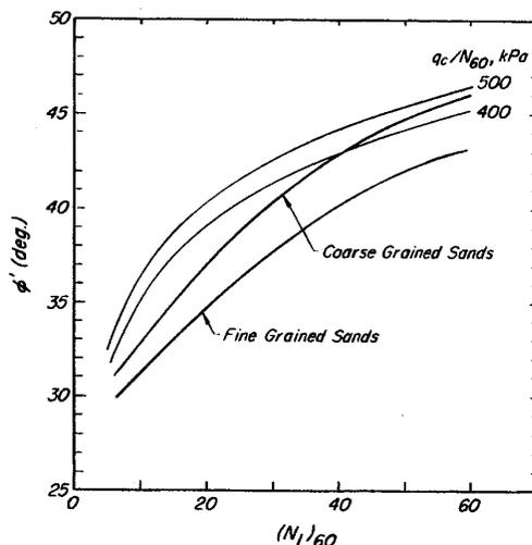
**Figure 7.5a. Empirical Correlation Between Friction Angle of Sand and Normalized Standard Penetration Blow Count (Terzaghi et al., 1996)**
