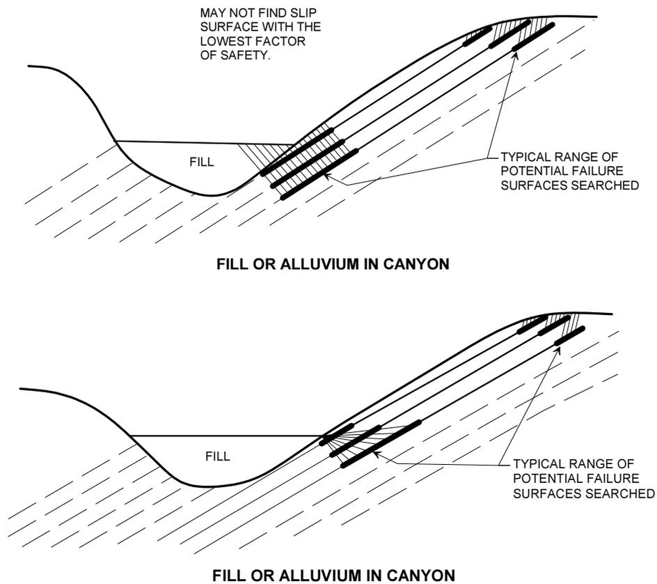
**Figure 9.1e. Failure Surfaces Combining Along-Bedding and Cross-Bedding Failure - Fill or Alluvium in Canyon (bottom diagram indicates correct geometries)**
