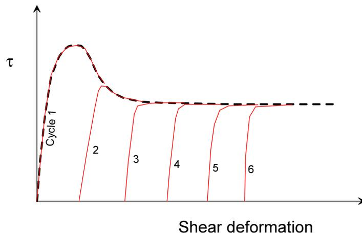
**Figure 7.6. Schematic of Multiple-Cycle Direct Shear Test Results**
